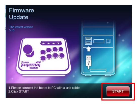
**STEP 4 DO NOT** disconnect the usb cable during the update process
